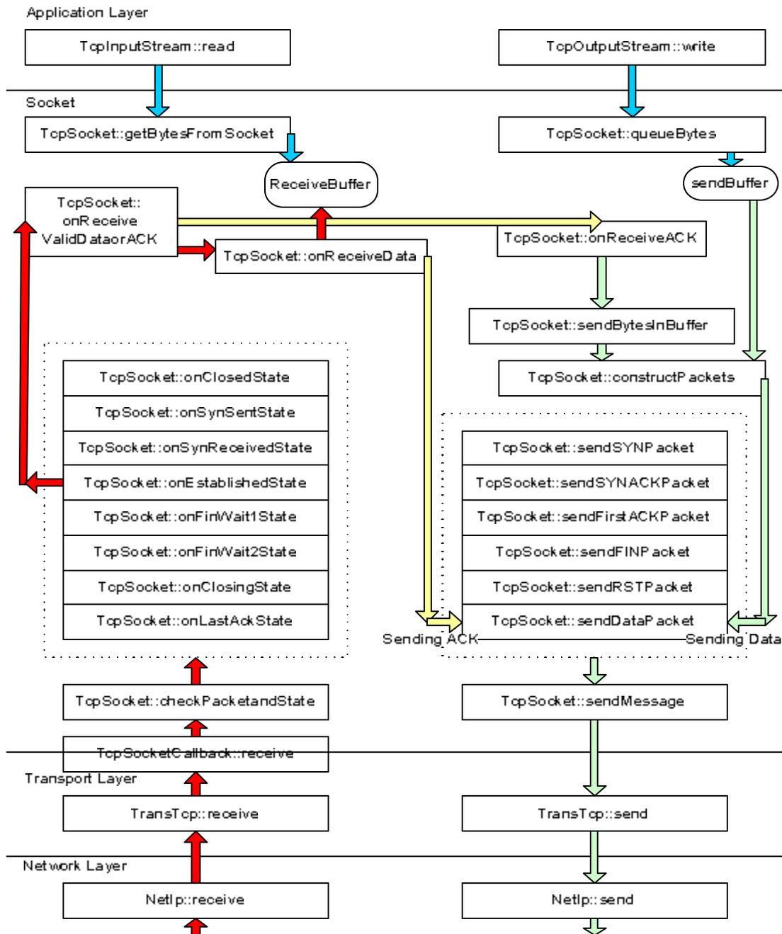
The arrows with red color indicates the execution flow when a packet is received. Then, in method `onReceiveValidDataorACK` in `TopSocket`, it is divided into 2 paths. The first path is when data packet is received (still in red). The second path is when ACK is received, denoted by yellow arrows. From the diagram, it can be observed that after receiving data, the arrow becomes yellow since TCP will send acknowledgement packet after receiving data.
