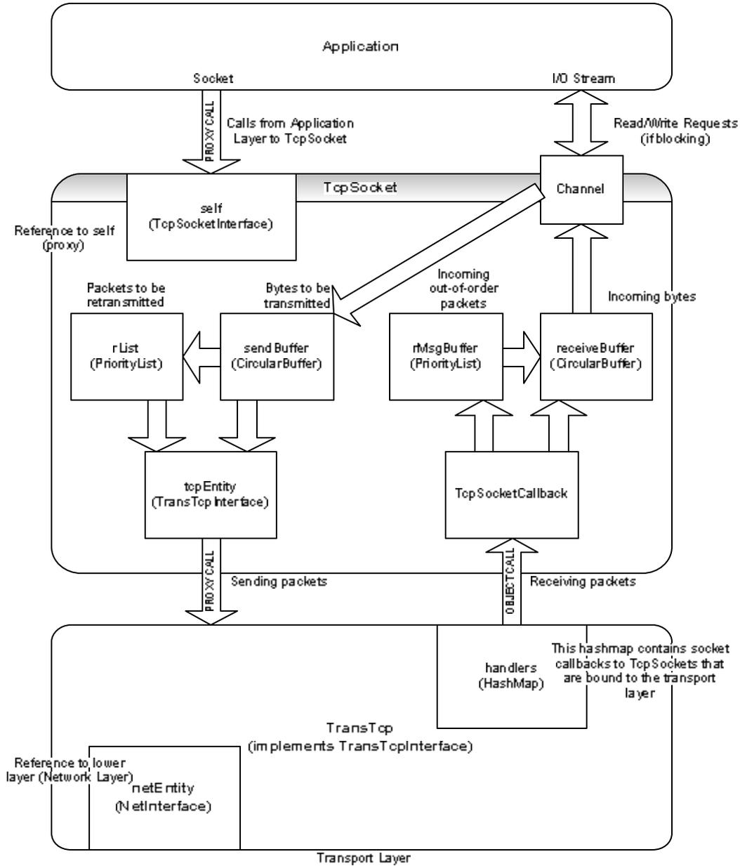
The next diagram explains the flow of the program during sending and receiving data and acknowledgement :
