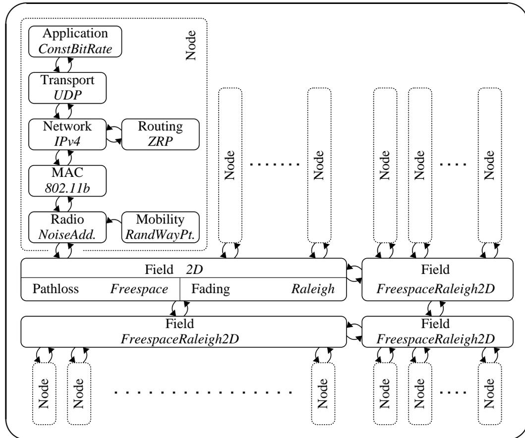
The SWANS simulator consists of event-driven components that can be configured and composed to form a meaningful wireless network simulation. Different classes of components are shown in a typical arrangement together with specific instances of component implementations in italics.
