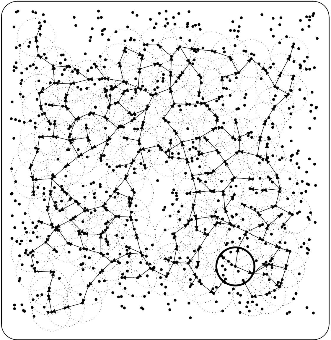
Figure 6.7: An example 800-node,  $R = 4$  bordercast plot
