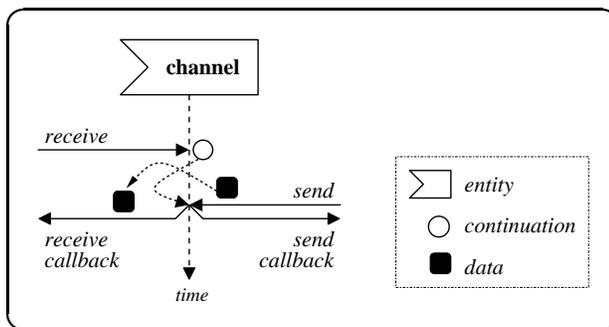
A blocking CSP channel is built using continuations. SWANS uses JiST channels to create simulated sockets with blocking semantics. Other simulation time synchronization primitives can similarly be constructed.
