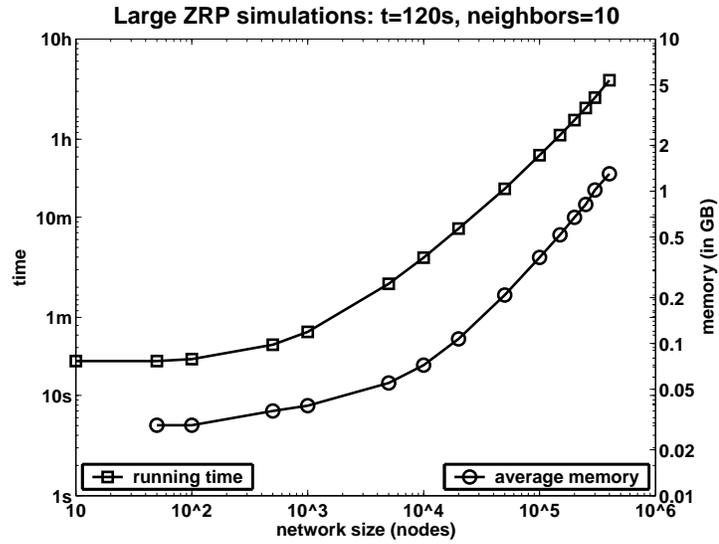
Figure 5.4: SWANS simulates up to 500,000 nodes at a density of 10 neighbors per node, each running ZRP, on a 2.8GHz machine with 4GB of memory.
