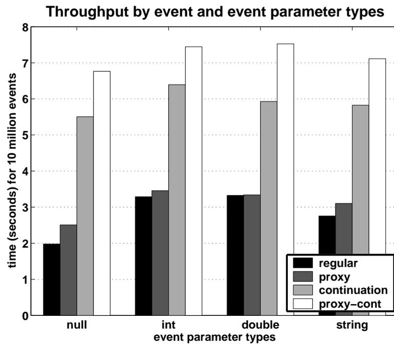
Figure 5.7: Manually boxing Java primitives for reflection-based invocation and unrolling the Java stack for blocking event continuations are Java-related overheads that could be eliminated from the performance-critical simulation event loop.
