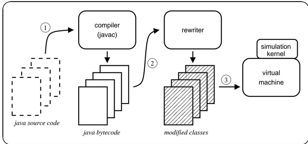
Simulations are (1) compiled, then (2) dynamically instrumented by the rewriter and finally (3) executed. The compiler and virtual machine are standard Java language components. Simulation time semantics are introduced by the rewriter and are supported at runtime by the simulation time kernel.
