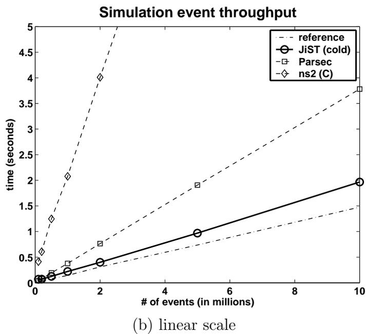
Figure 5.5: JiST has higher event throughput and comes within 30% of the reference lower bound program. The kink in the JiST curve in the first fraction of a second of simulation is evidence of JIT compilation and optimization at work.
