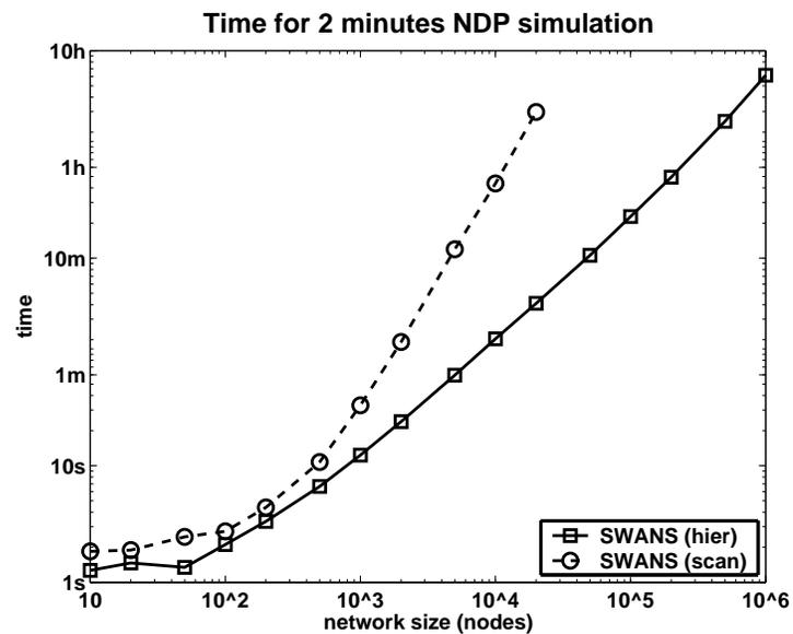
Figure 5.3: SWANS scales to networks of  $10^6$  wireless nodes. The figure shows the time for a sequential simulation of a node discovery protocol in a wireless ad hoc network running on a commodity machine.
