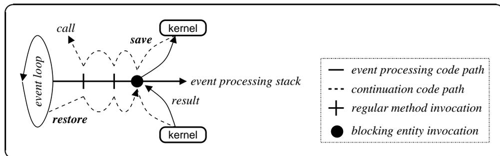
The JiST event loop also functions as a continuation trampoline. It saves the continuation state on a blocking entity method invocation and restores it upon receiving the callback. Due to Java constraints, the stack must be manually unwound and preserved.
