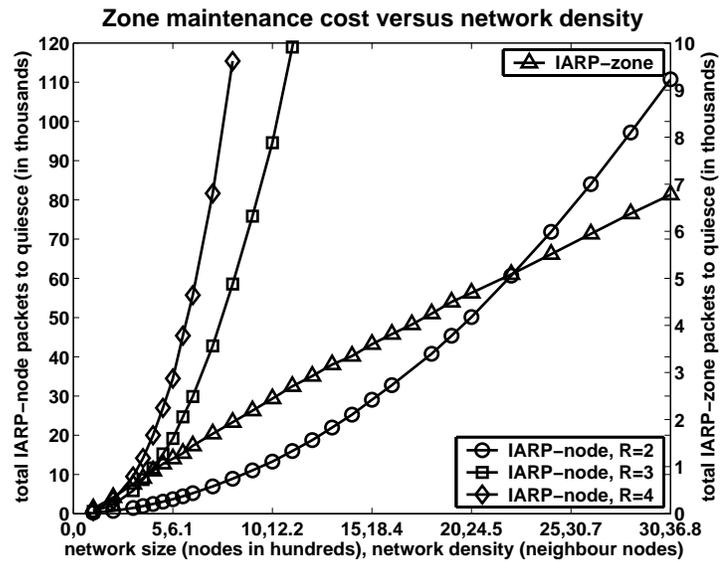
Figure 6.8: Cost of zone maintenance increases dramatically with increased density and zone radius.
