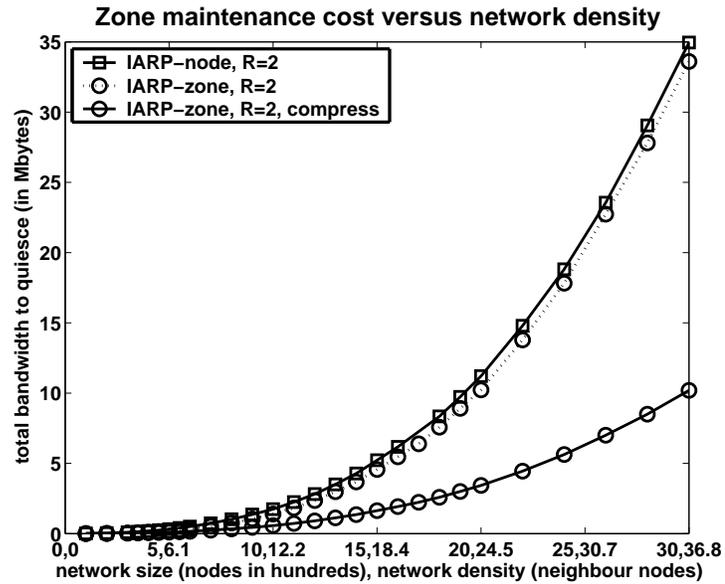
Figure 6.10: Comparing the two zone maintenance protocols shows that zone-wide link update aggregation and efficient encoding is beneficial.
