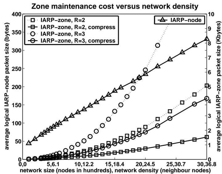
Figure 6.9: Aggregated link state can be encoded efficiently to reduce average size of update packets.
