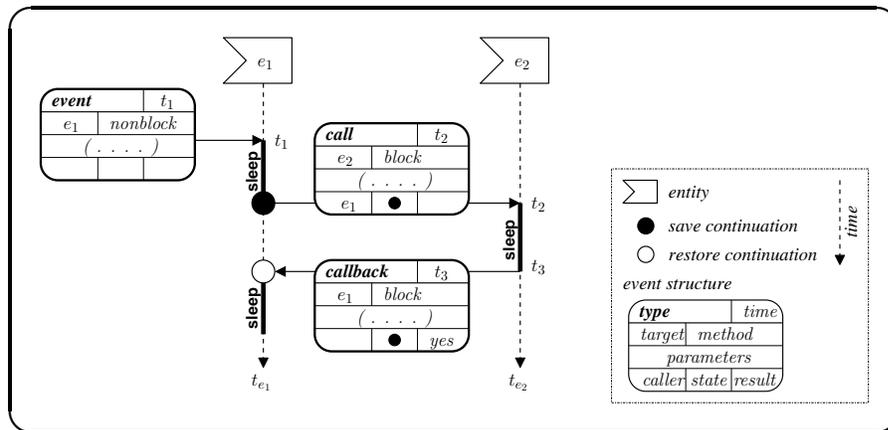
Blocking events allow process-oriented development. When a blocking entity method is invoked, the continuation state of the current event is saved and attached to a call event. When this call event is complete, the kernel schedules a callback event to the caller. The continuation is restored and the caller continues its processing from where it left off, albeit at a later simulation time.
