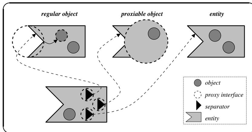
Proxy entities use an interface-based approach to identify entity methods, thus simplifying the development of entities. The proxy system call behavior depends on the type of the target.
