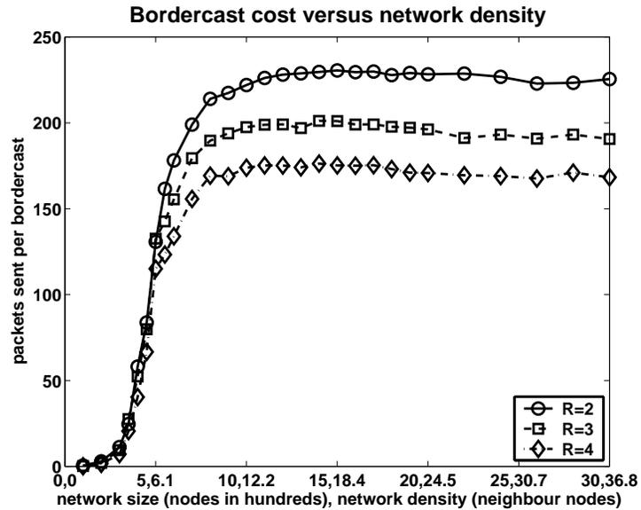
Figure 6.5: Increased zone radius improves bordercast performance, primarily due to edge effects.
