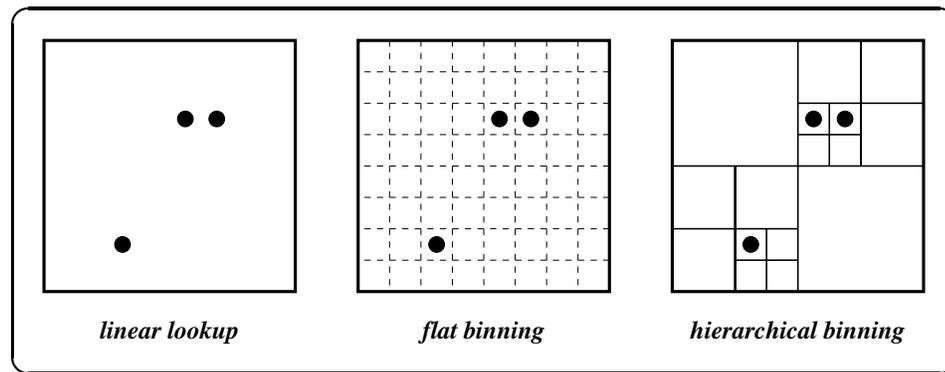
Efficient signal propagation is critical for wireless network simulation performance. Hierarchical binning of radios on the field allows location updates to be performed in expected amortized constant time and the set of receiving radios to be computed in time proportional to its size.
