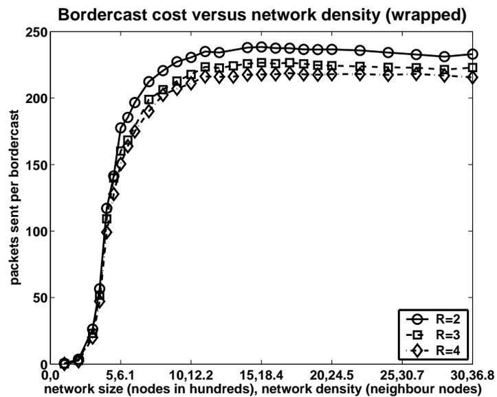
Figure 6.6: Discounting edge effects, bordercast cost is not significantly affected by increased zone radius.
