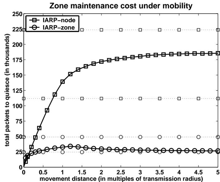
Figure 6.11: Mobility increases the cost of zone maintenance.
