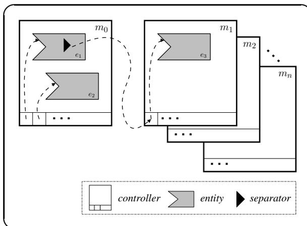
The JiST framework allows parallelism to be transparently introduced by partitioning the system entities among different, possibly distributed, threads of control. Separators preserve the single system image abstraction among distributed controllers.
