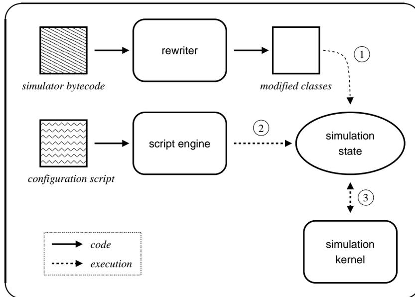
JiST provides multiple scripting interfaces to configure its simulations without source modification, memory overhead, or loss of performance. (1) As before, simulation components are loaded and rewritten on demand. (2) The script engine configures the simulation via reflection and may dynamically compile scripts to bytecode for performance. (3) The simulation runs as before, interacting with the kernel as necessary.
