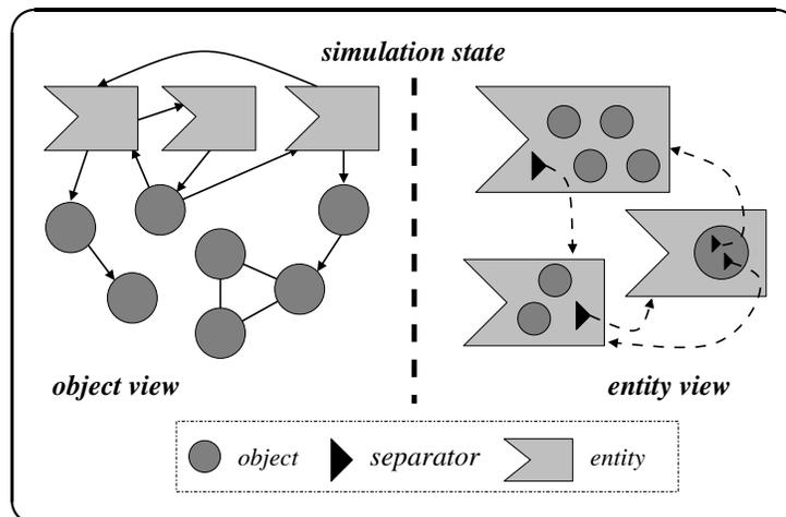
(b) At runtime, entity references are transparently replaced with separators, which both preserves the separation of entity state and serves as a convenient point to insert functionality.
