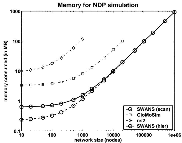
Figure 5.2: SWANS can simulate larger network models due to its more efficient use of memory.
