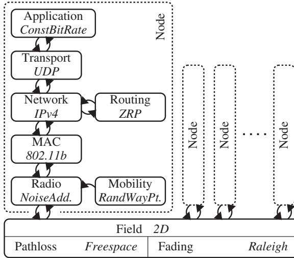
**FIGURE 19.1** The SWANS simulator consists of event-driven components that can be configured and composed to form wireless network simulations.
