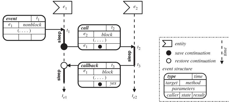
**FIGURE 19.7** The addition of blocking methods allows simulation developers to regain the simplicity of process-oriented development. When a blocking entity method is invoked, the continuation state of the current event is saved and attached to a call event. When this call event is complete, the kernel schedules a callback event to the caller. The continuation is restored and the caller continues its processing from where it left off, albeit at a later simulation time.
