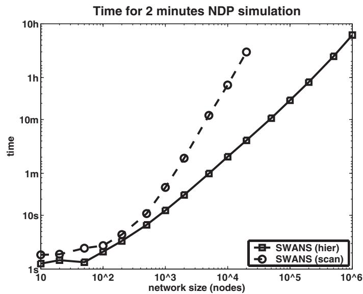
**FIGURE 19.6** SWANS scales to networks of  $10^6$  wireless nodes. The figure shows the time for a sequential simulation of a heartbeat NDP.
