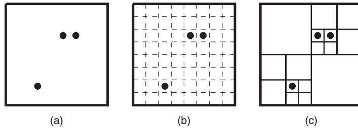
**FIGURE 19.4** Hierarchical binning of radios in the coverage area allows location updates to be performed in expected amortized constant time and the set of receiving radios to be computed in time proportional to its size. (a) linear lookup, (b) flat binning, and (c) hierarchical binning.
