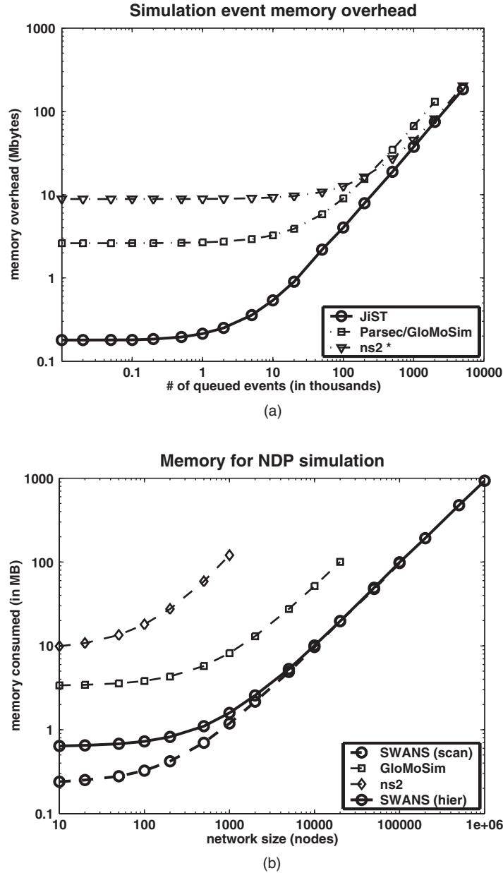
**FIGURE 19.5** JiST allocates entities efficiently: comparable to GloMoSim at 36 bytes per entity and over an order of magnitude less than Parsec or ns2. SWANS can simulate correspondingly larger network models due to this more efficient use of memory and more sophisticated memory management protocols enabled by the garbage collector.
