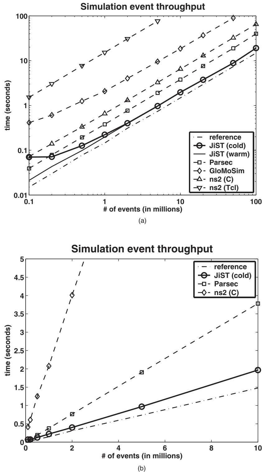
**FIGURE 19.2** JiST has higher event throughput and comes within 30 percent of the reference lower bound program. The kink in the JiST curve in the first fraction of a second of simulation is evidence of JIT dynamic compilation and optimization at work.
